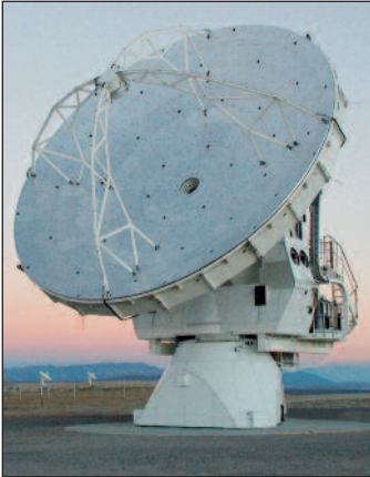
The ALMA project in the Atacama desert in Chile is to include up to 64 antennas interconnected to form an enormous radio telescope. PI Hexapod systems are used to position the secondary reflectors in the antennas. The M-850K systems, specially designed for outdoor operation in hostile conditions, can position loads of up to 75 kg (photo: Vertex Antennentechnik GmbH)
